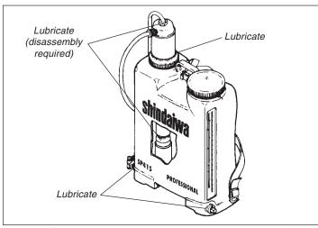
Periodically clean and lubricate the pump chamber and actuating linkage with a high quality lithium grease.
